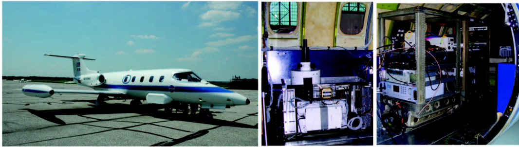
Fig. 1. (Left) NASA Glenn Lear-25 aircraft. The nadir window assembly is just below the NASA logo. Photographs of the lidar installed on the aircraft showing the sensor head assembly (middle) and the dual aircraft racks (right).
