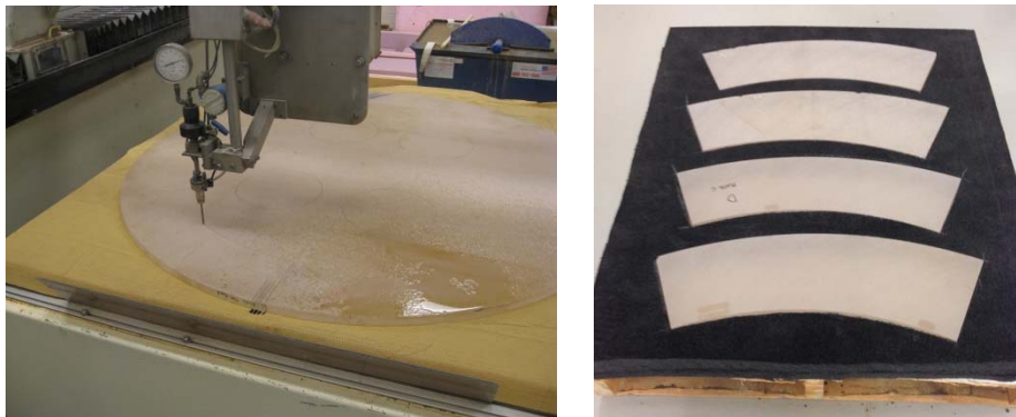
Figure 18 – One of the AMTD mirror plates (face sheets) being rounded in AWJ (left) shown with residual glass sent to Ormond (right)
