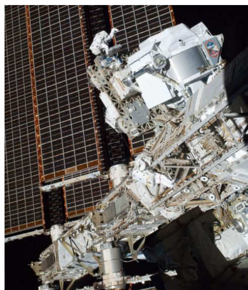
Figure 2. NICER/SEXTANT will be mounted to ELC2, approximately where the EVA crew member is shown.
