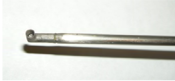
Figure 2.14: Fast-response total pressure probe.
