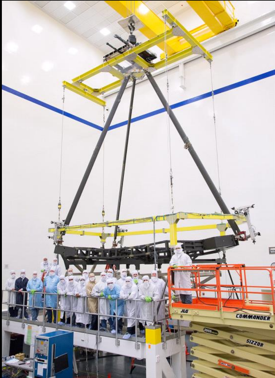
Pathfinder secondary mirror structure deployment test
