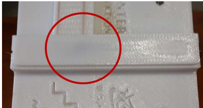
Figure 16: Light discoloration observed at wire junction due to arcing
