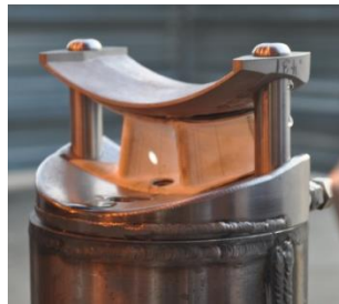
Vane doublet with temperature sensing coating in test fixture.
