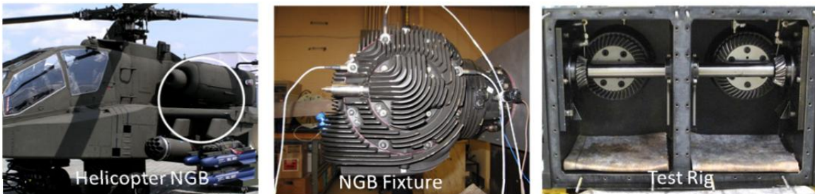
Figure 2.—Three spiral bevel geared systems.
