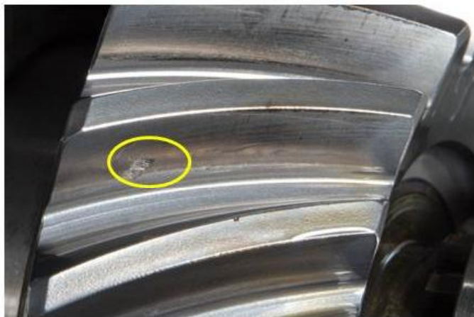
Figure 16.—Damage to one pinion tooth.
