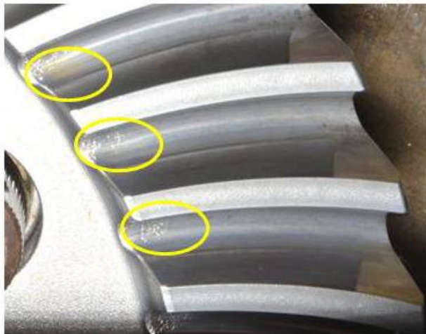
Figure 14.—Gear teeth anomaly on the second gear set.
