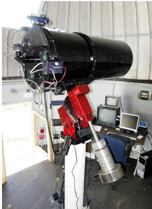
Figure 1. The 0.5-m RCOS Ritchey-Chrétien telescope used for lunar impact monitoring at the ALaMO. This telescope worked in conjunction with another located at the ALaMO and one at WCO.
