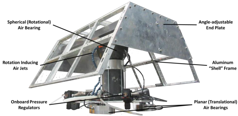
Figure 4. Reconfigurable Reactive Spacecraft (Orbital Object) Simulator
