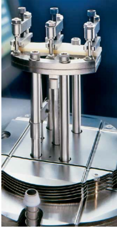
Figure 4. A rectangular material sample ( \approx 2.5 in \times 0.5 in \times thickness) mounted and clamped horizontally in the DMA with a cantilever clamp used in the dual cantilever mode. A torque wrench was used to tighten screws at all three points with a torque value appropriate for the material stiffness tested.
