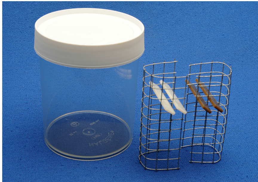
Figure 3. 1000-mL Nalgene plastic jar (left) used to contain flexible wire racks for containing up to 18 DMA samples per rack, and two wire racks containing samples of two different materials (right) were immersed in one solution (pretreated urine or brine solution) per jar. Each jar was hand-tightened and stored in a fume hood at room temperature until samples were removed for DMA testing.
