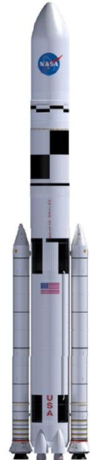
Figure 7. SLS Block 1B with EUS and 8.4m PLF. (Image credit: The Boeing Company)
