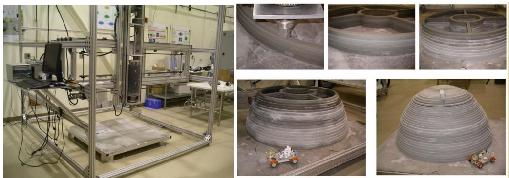
Figure 1 – Contour Crafting Machine at NASA/MSFC and Typical Fabricated Structures
