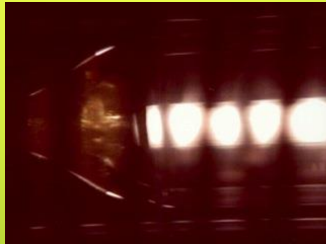
Growth Interface of Crystal A in Space at Different Time
