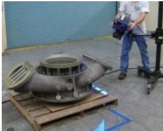
Structured light scanning the Mk-10A fuel inlet
