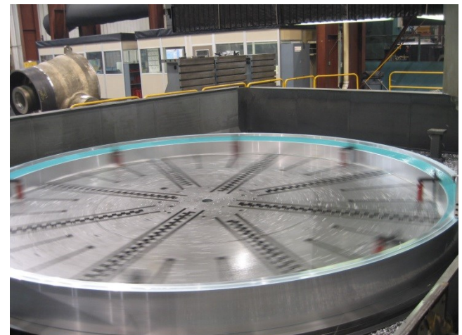
Dynetics y-ring in machining
