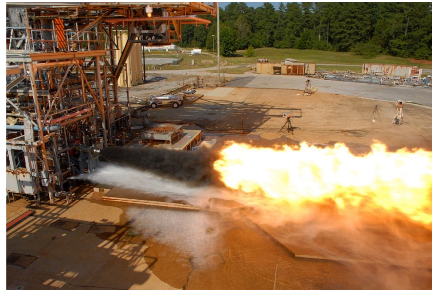
F-1B SLM GG injector hotfire test at NASA MSFC
