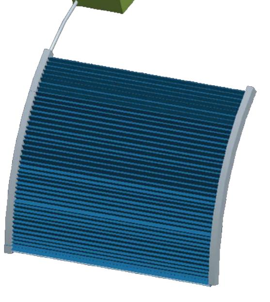
"Thirsty Walls" provide gentle, passive contact between ventilation air and Air Revitalization functions of temperature control, relative humidity control, and CO<sub>2</sub> removal.
