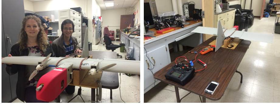
(a) PI Kristin Yvonne Rozier and Ph.D. Research Intern Quoc-Sang Phan assembling a DragonEye on the test stand in December, 2015. (b) DragonEye in a test stand flight test, with motors running, without fan. For tests with a fan, the large fan was placed on a table in front of the test stand.
