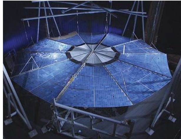
Figure 9. Engineering development unit circular solar array from Manzella and Hack. 2
