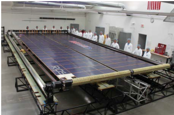
Figure 8. Engineering development unit roll-out solar array from Manzella and Hack. 2
