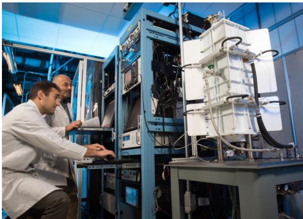
Figure 2. The ASRG EU2 under test in NASA GRC's Stirling Research Laboratory.
