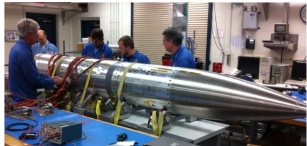
Figure 7. Integration of RCHS test section into rocket.
