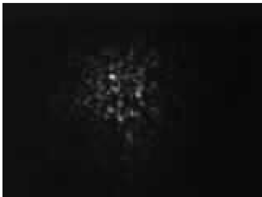
Figure 3 Snapshot of QCL beam through prepared phase plate
