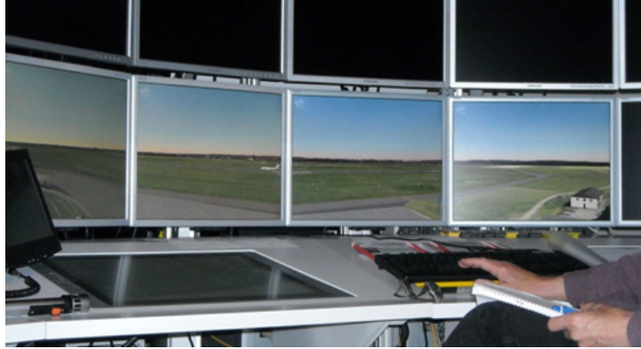
Figure 2. Participant at a simulation console judging the outcome of a landing aircraft just after touchdown (2 nd monitor from left). Approach on the rightmost monitor, touchdown is on the left side of second monitor from the right. Reconstructed panorama compressing the 180°-tower view to ca. 120° for subjects at the RTO-console.
