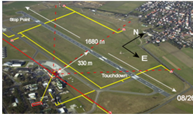
Figure 1. Aerial view of Braunschweig airport showing the circled location of the simulated (and real) cameras, fields of view of the four cameras (radial sectors), and some dimensions and reference points.
