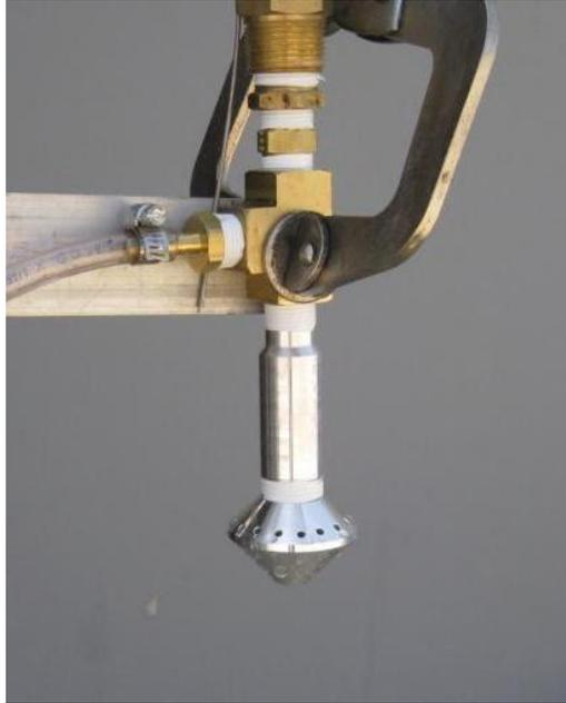
Figure 4.—Inlet diffuser.
