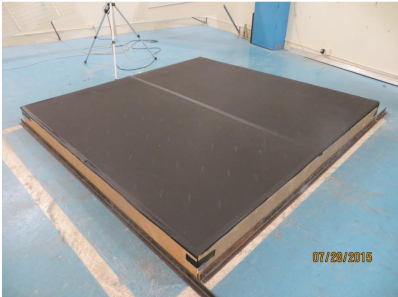
Figure 2. RAL's Absorption Test Setup (8-in. thick ML ULb with Soundtex ® Cover Sheet with Sealed Edges, ASTM C423 Reverberation Room Method).
