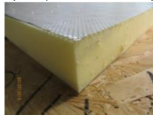
Perforated Mylar® Coversheet with ML ULb foam
