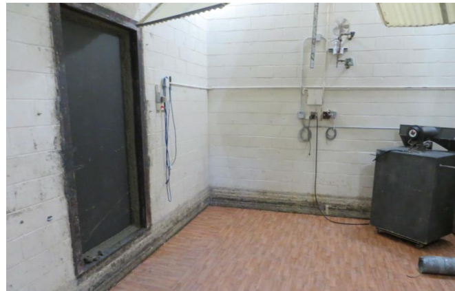
Figure 9. RAL's Test Setup for Transmission Loss (TL) Testing (ASTM E-90 Airborne Sound TL for Building Partitions and Elements Method).
