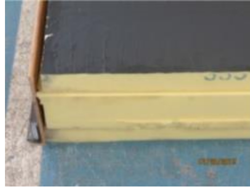
Un-reinforced Kapton® Coversheet with ML ULb foam
