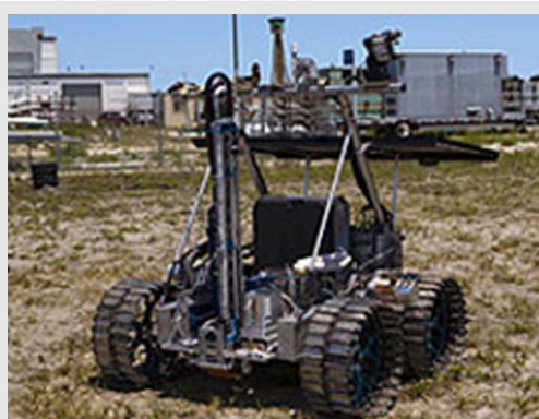
The RESOLVE's main tool is a drill designed to burrow about one meter into the lunar soil to extract water. Photo credit: NASA/Dmitri Gerondidakis
