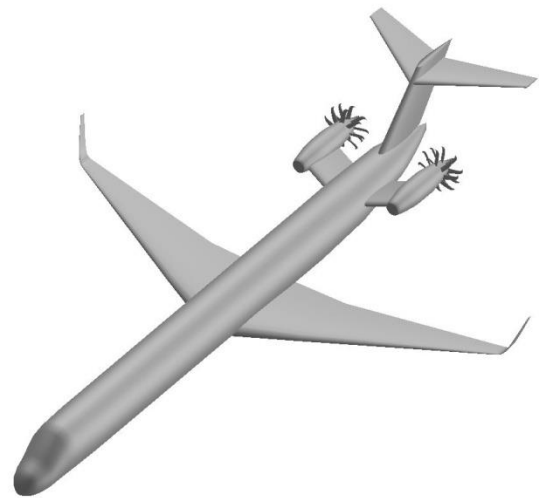
Figure 2. NASA’s notional, advanced single-aisle transport airplane equipped with fuselage-mounted open rotor engines.
