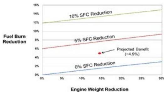
**Figure 1: Regional jet fuel burn sensitivities showing reduction in fuel burn and engine weights.**
