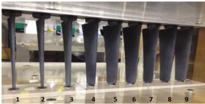
**Figure 4: Inlet Guide Vane Cascade Test Section**
