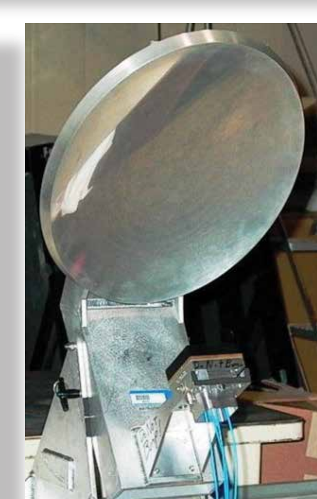
WISM reflector antenna with WISM antenna feed.
