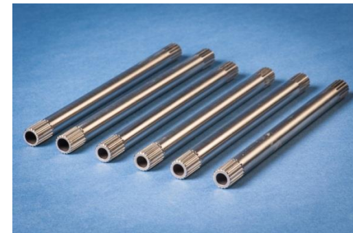
Successful hot extrusion (rods and tubes)
