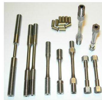
Successful hot extrusion (rods and tubes)
