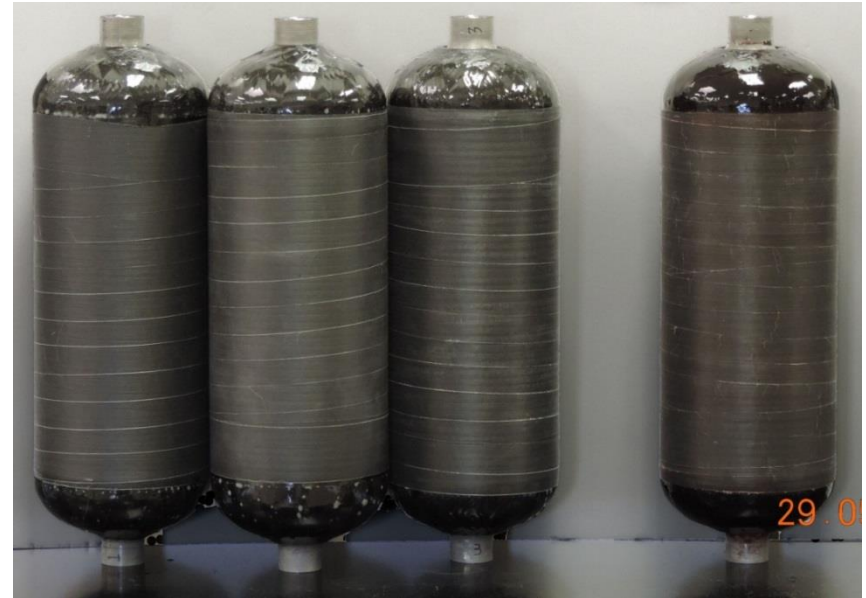
Epon 828 Resin with Huntsman T-403 Curing Agent
