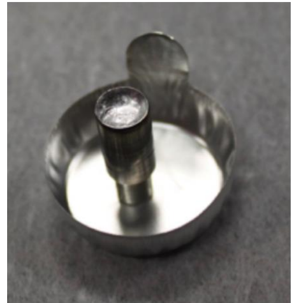
Quench vessel filled with a gallium-indium alloy
