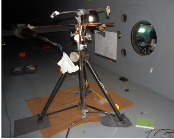
Figure 4. Calibration plate installed in test section. Figure 5. Applying speckles to Performance model.
