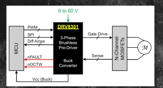
Three-phase gate driver IC Hand-shaking to prevent current shoot-through Current shunt amplifiers for low-side current measurement Already have code that works with the chip
