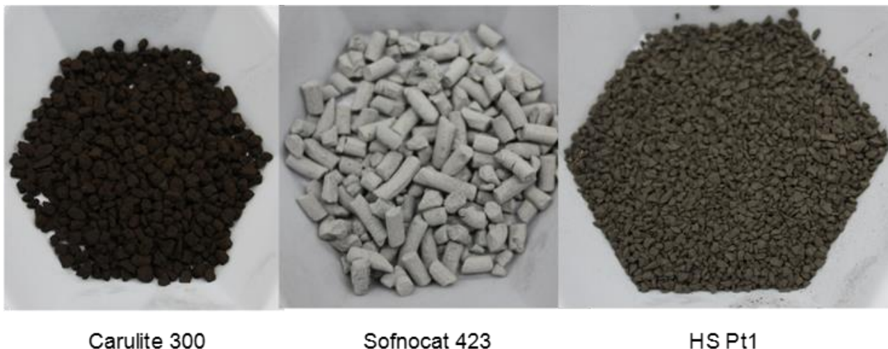
Figure 1. Three low temperature oxidation catalysts for removal of CO from spacecraft gas streams were evaluated for operation at 40% humidity.
