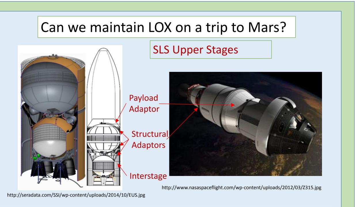
The largest source of heat to LOX and LH2 tanks in orbit is conduction from warm attached structures (e.g. the stage adaptors and interstages). If a cryogenic selective surface could be put onto these external surfaces, lowering their temperature, then propellant boil-off could be substantially decreased (credit to Wesley Johnson at GRC).
