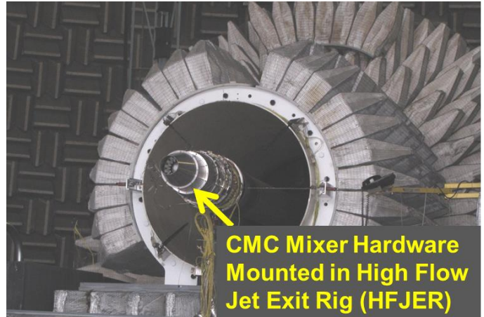
Figure 7: Nozzle Acoustics Test Rig, with CMC hardware mounted
