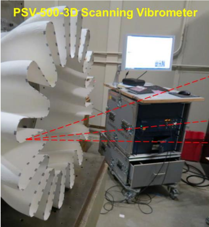
Figure 12: Laser vibrometry was performed on CMC Mixer 2014 while it was attached to the mount plate. A small impact hammer was used to excite the modes
