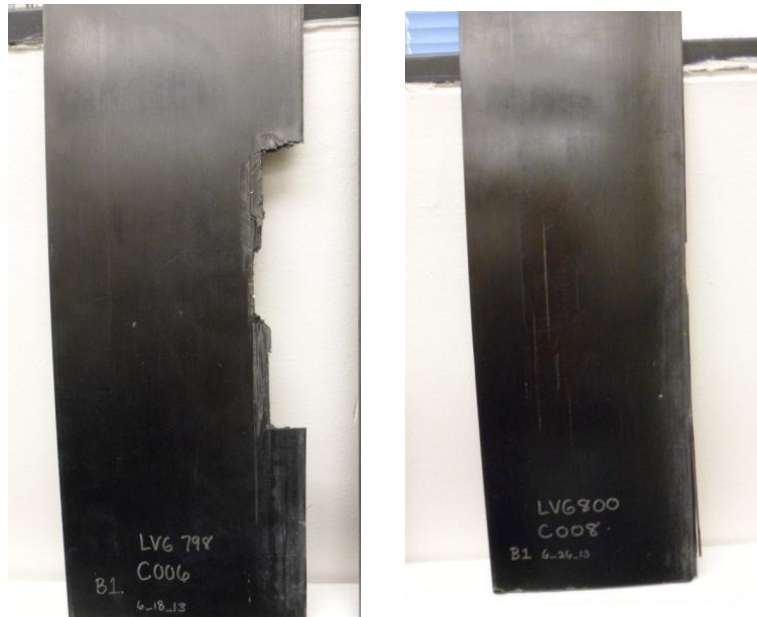
Figure 9. Photos of baseline (left) and toughened (right) panels after impact
