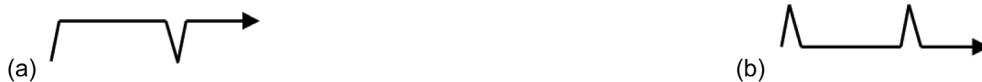
Figure 4.—The two dwell cycles utilized for the NLCF testing. (a) Max dwell: 1.5-90-1.5s. (b) Min dwell: 1.5-1.5-90s.
