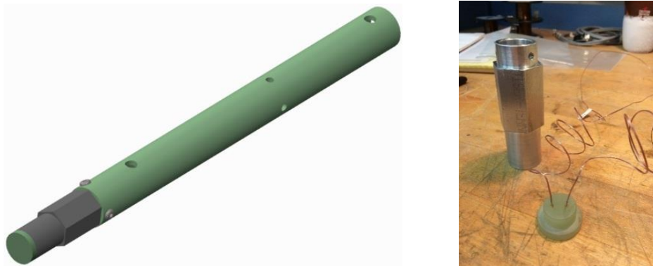
Figure 4. Compression piston assembly (left); and piston head, G10 face, and embedded thermocouples (right).
