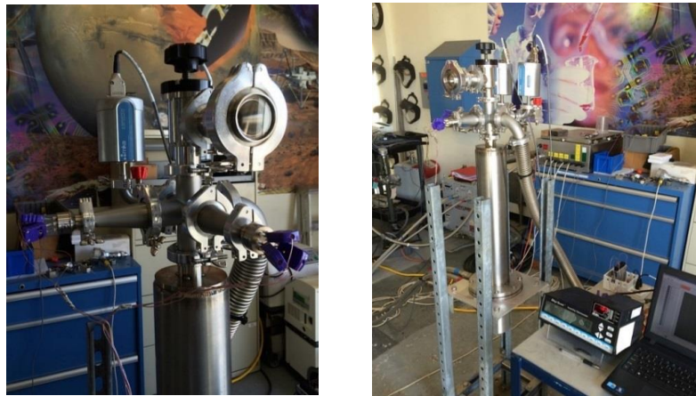
Figure 1. Apparatus for Low-Temperature Training of Materials (ALTM): actuator and upper feed-through (left); overall view with cryocooler in background, and data acquisition in foreground (right).
