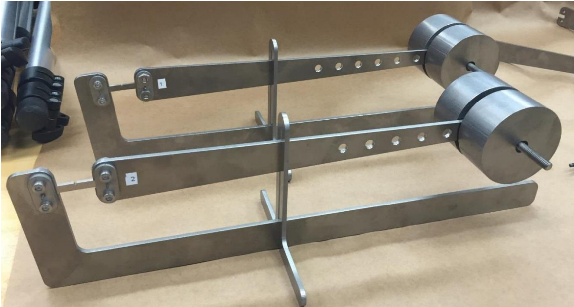
Figure 8. ASTM E1681 loading fixture. SE(B) specimens were incrementally loaded until failure.
