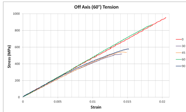
Figure 8. Measured elastic moduli and strengths from the off-axis coupon tests of T700/PR520.
