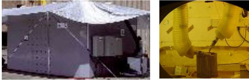
Figure 12. SHARS Mobile Hot Cell Unit with Interior Remote Manipulator Arms
