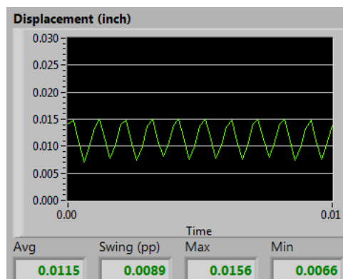
Figure 35: Time response (in seconds) of spool position under a 1,000 Hz excitation
