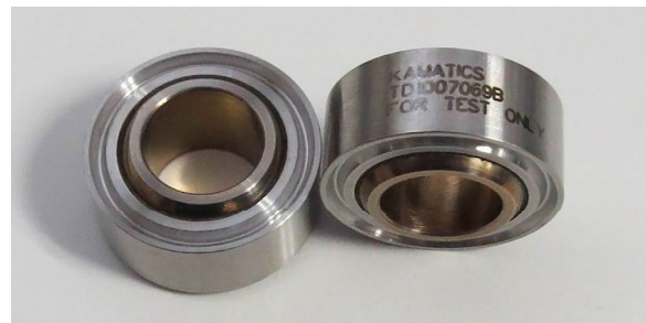
Figure 3.—Test bearings that utilize spherical inner race drilled balls made from 60NiTi.
