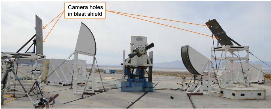
Figure 18.—High-speed camera locations for digital image correlation; four cameras, two per panel.
