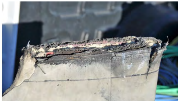
Figure 10.—Blade section at cut line.
