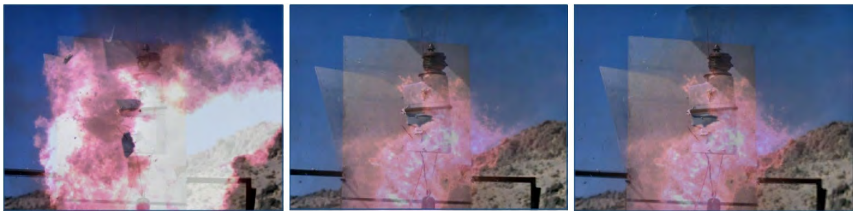
Figure 9.—Shape charge detonation, full-circumference configuration.
