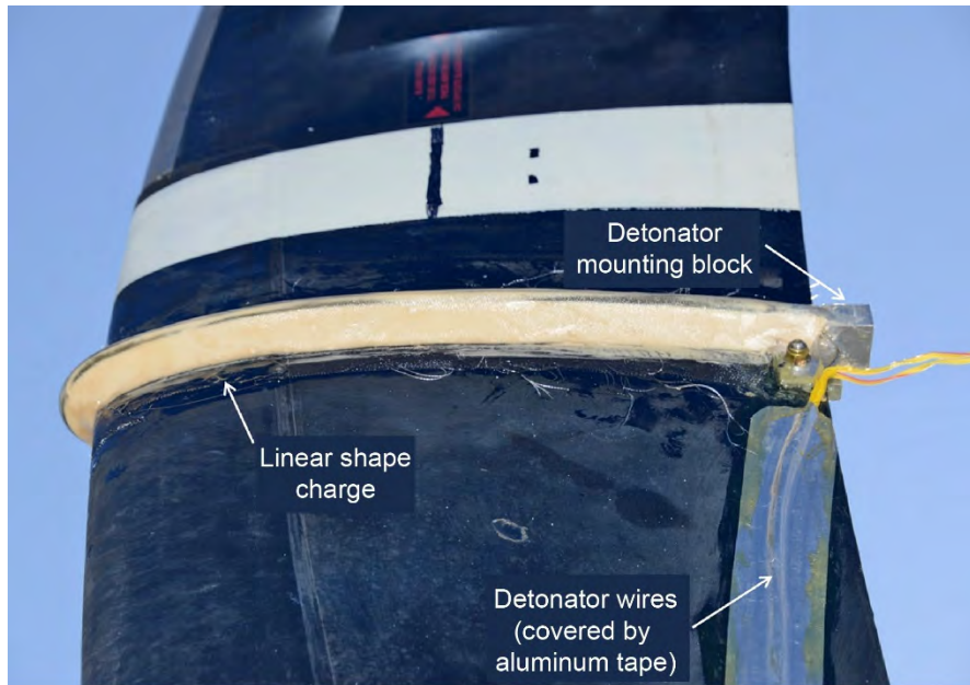
Figure 27.—Linear shape charge final installation.
