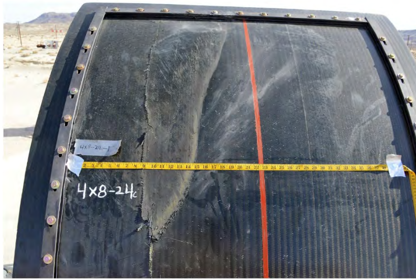
Figure 36.—24-ply composite panel postimpact damage, front side.
