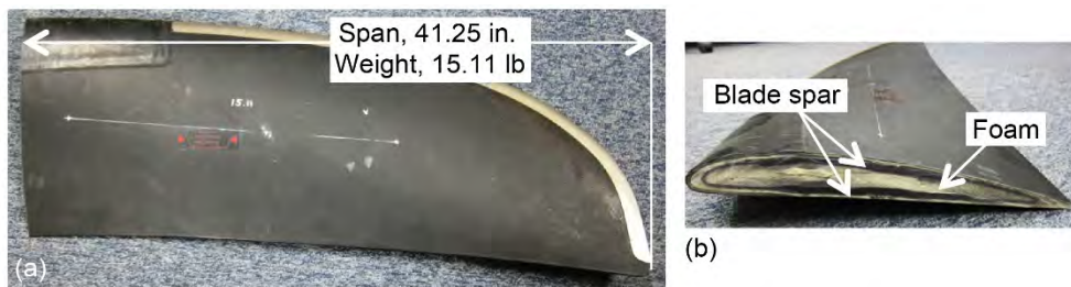
Figure 5.—Candidate blade configuration for shield impact. (a) Outer blade length and weight. (b) Blade cross section.
