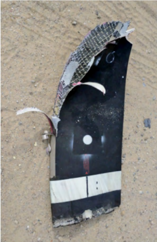
Figure 40.—Upper blade after impact on 24-ply composite panel.
