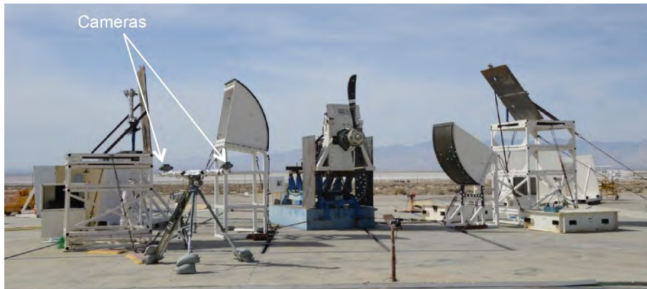
Figure 23.—Cameras used to measure blade kinematics.
