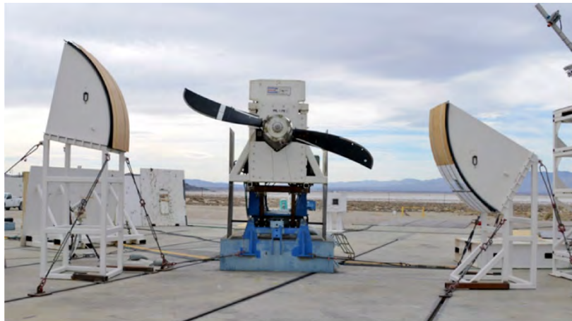
Figure 6.—Spin rig on T406 spin fixture.
