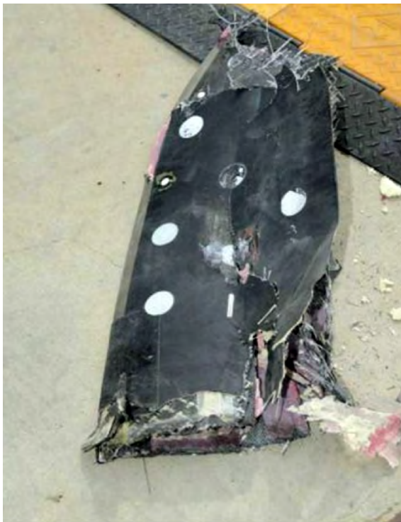
Figure 34.—Lower blade after penetration of 20-ply composite panel.
