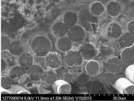
Micrograph of SiC/SiC composite showing oxidized BN fiber coating. Courtesy of Ram Bhatt (NASA/GRC).
