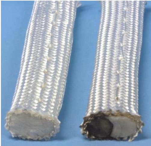
Compliant Thermal Barriers (CTB's)
