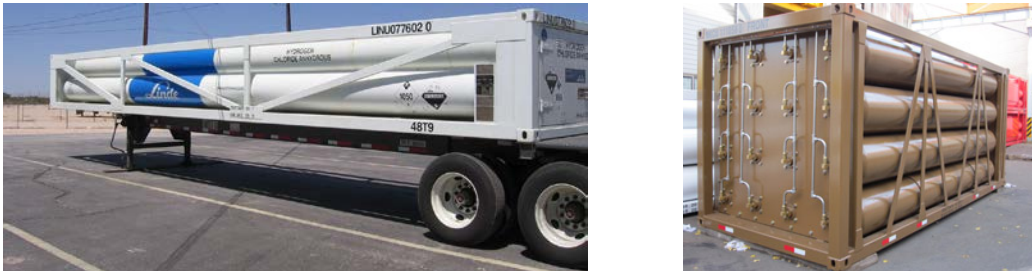
Figure 6. Example of a tube trailer (left) and tube bank (right).
