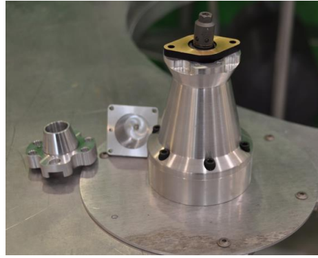
Launch Lock Post Components
