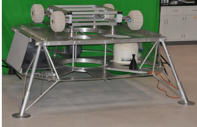
Test configuration of mock up lander with mock rover supported by Launch Locks
