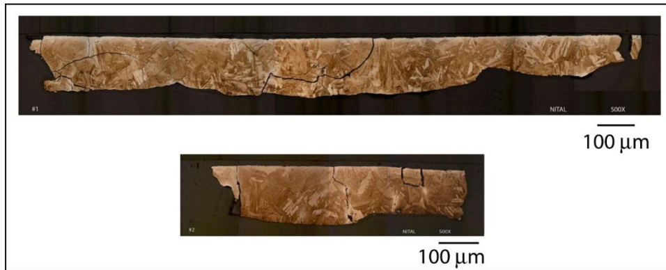
Figure 13. Etched starboard SARJ fragment showing transgranular crack propagation and fracture within the nitride case of the 15-5 PH race surface. Credit: P. Marciniak & B.
