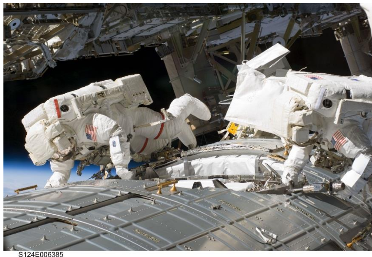
Figure 15. Astronauts Mike Fossum and Ron Garan testing a grease gun specifically designed to aid in cleaning of the starboard SARJ race ring debris. Credit: NASA
