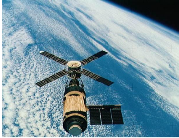
Figure 1. Skylab orbiting the Earth, as seen by a departing crew capsule after one of the long-duration missions. The parasol-like repair shield is seen at the bottom of the image, a fix that enabled mission and program success.
